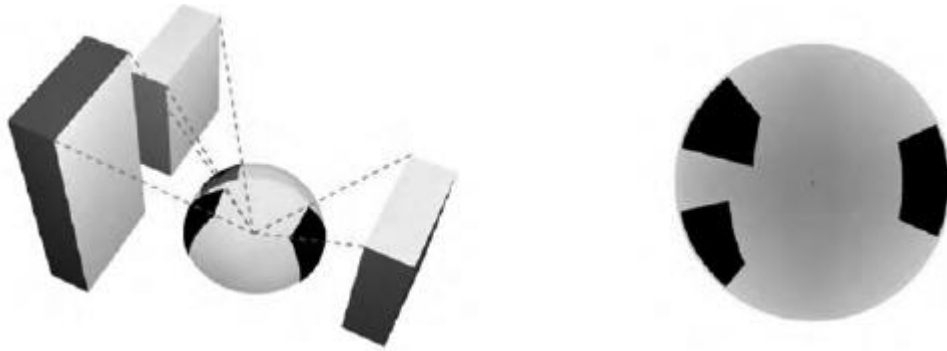
Figure 12.1.10 Sky View Factor means the extent of sky observed above a point as a proportion of the total possible sky hemisphere above the point
